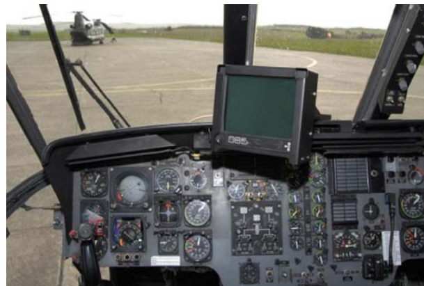
Figure A-2: Imaging Sensors and Pilot's Panel-Mounted Display.
