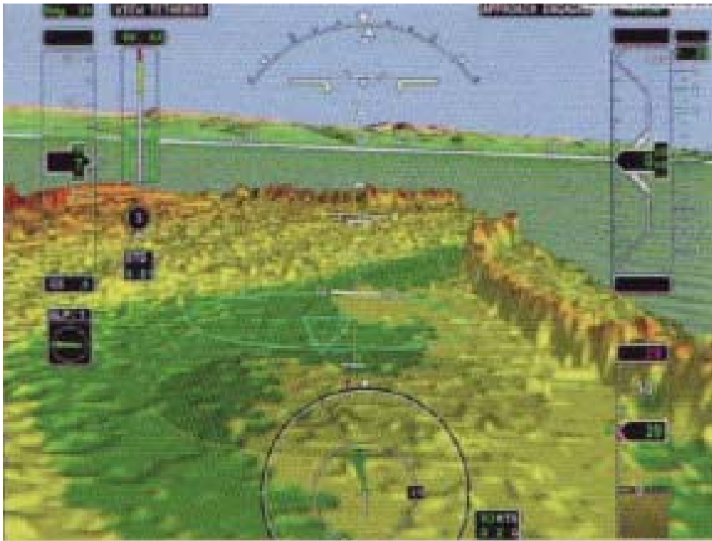
Figure A-7: Sandblaster Display Includes Radar Data (Close) and Pre-Stored Terrain Elevation Data (Far) and Symbology.
