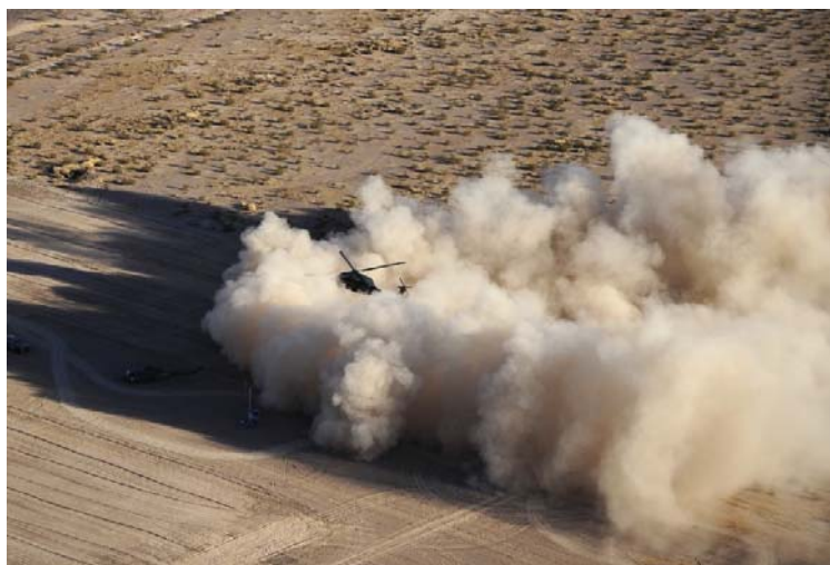
Figure C-16: Lanes were Plowed to Increase Quantity of Dust (EH-60L shown).
