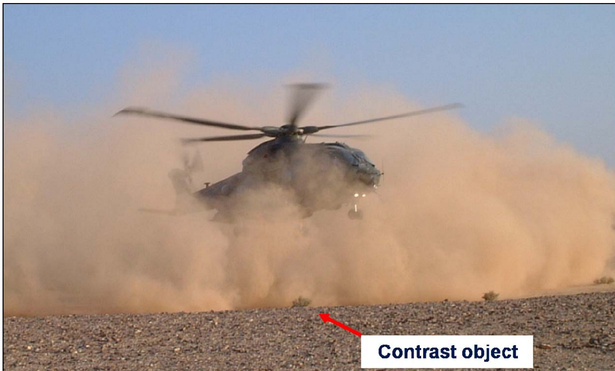
Figure 2-2: Helicopter Entering a Brownout Condition.
