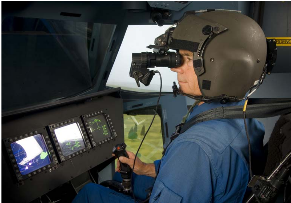
Figure A-12: NASA-Ames Vertical Motion Simulator with Panel-Mounted Displays and NVG-HUD.
