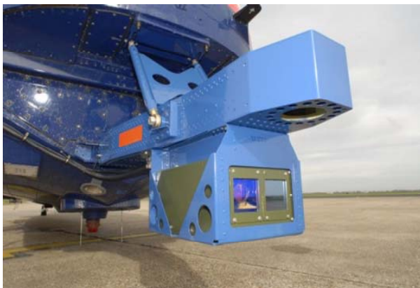
Figure A-2: Imaging Sensors and Pilot's Panel-Mounted Display.
