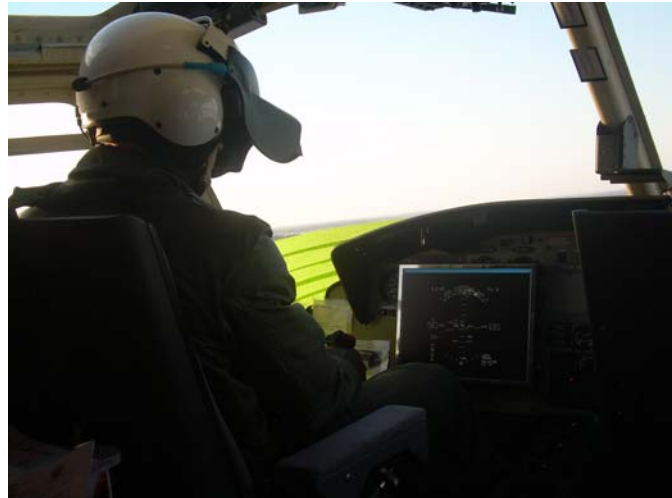
Figure A-20b): Pilot Flying Approach Using BOSS Display with Hood to Obscure the Out-the-Window View.
